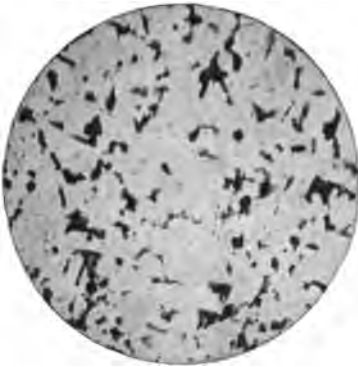
Fig. 11. Ferrite and Pearlite; Carbon, 0.16 Per Cent
